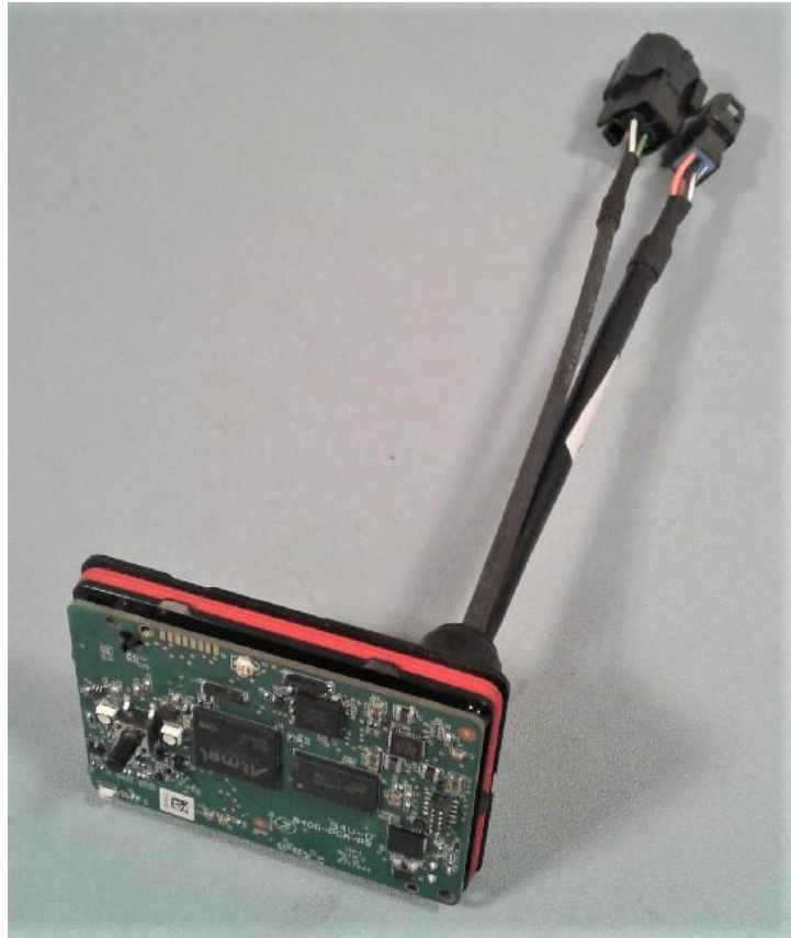
CCU Front Cover Removed View
